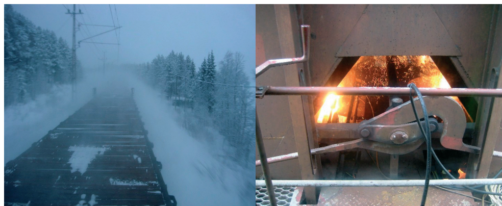
Figure 3.2.3: Testing braking performance under winter conditions and locked brake testing. Both are part of the homologation testing. Work is going on to enable the testing of these properties on test benches.
