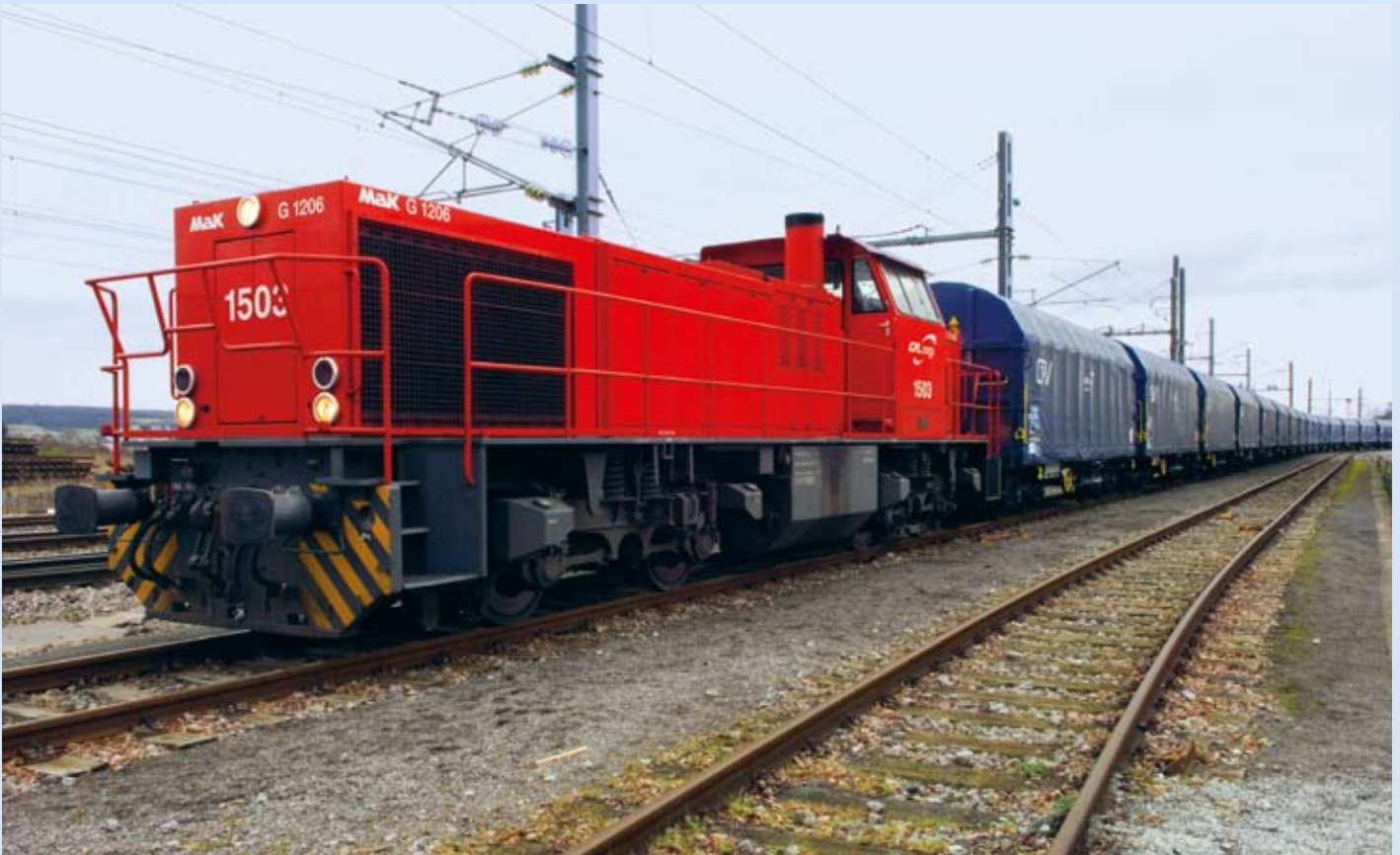
A Shimmns train – specially designed for the transport of steel coils, and covered to protect the coils from bad weather – in Pétange, Luxembourg.
